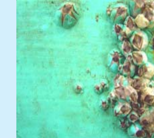
Figure 5c. A dynamic test panel with sufficient erosion of coatings to allow barnacles to attach and push out of the coating. Dynamic test may cause sufficient depletion of the antifoulant to create microscopic damage, which in turn allows barnacles to attach and eventually damage the coating.
