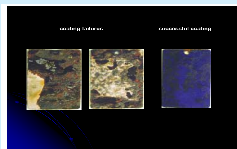
Figure 5a. Example of coating defects seen when panels were subjected to PDTS after 2 months of dynamic test.
