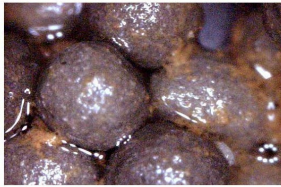
TYPICAL CERAMIC PROPPANTS WITH BACTERIAL BIOFILM
