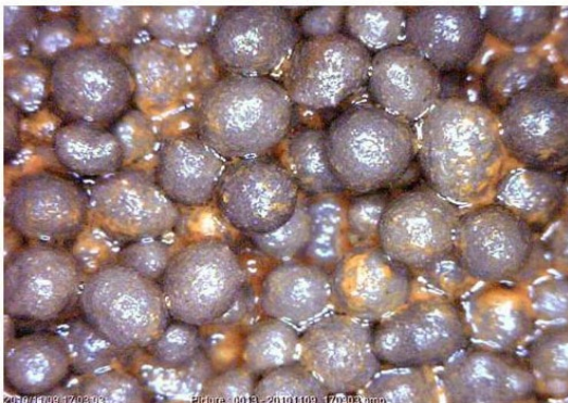
TYPICAL CERAMIC PROPPANTS WITH BACTERIAL BIOFILM
