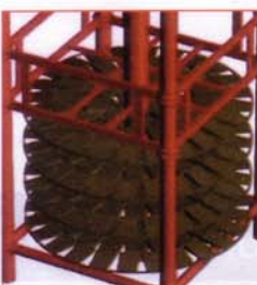
Figure 2. Diagrammatic representation of the rotating discs of the Poseidon Dynamic Test System. The rotating unit is completely submerged in seawater under the floating platform
