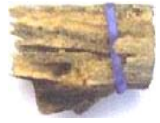
Fig. 22b. Wood sample treated with MR-08. (The blue band is for identification purposes only).
