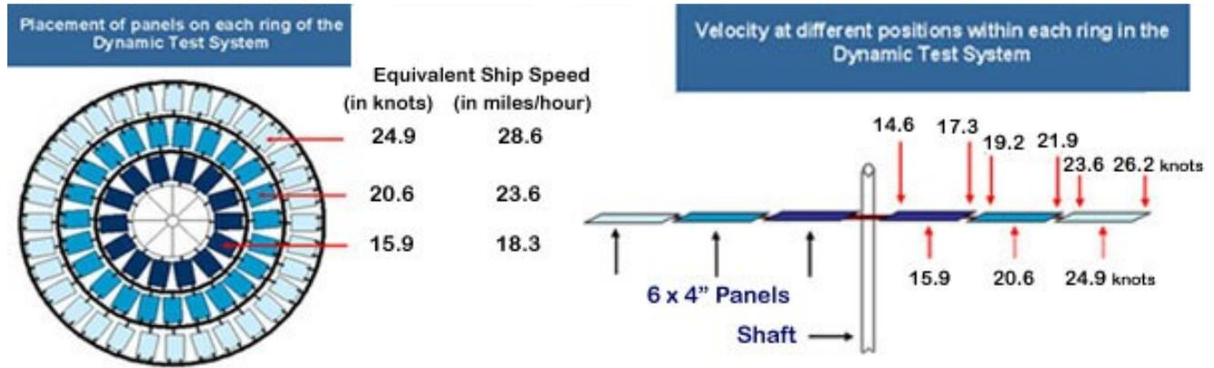
Since the test platform, supplied with power through underwater electric cable, is in the open sea under tropical conditions, the tests can be undertaken on a year round basis. This is particularly useful test paradigm to measure the performance of a smooth surface in shedding barnacles off the surface when subjected to different speed.
