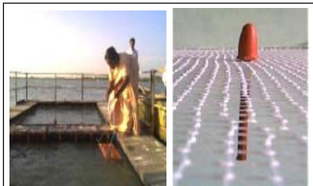
Figure 6. Typical method of hanging the painted rods and placement of the test series on the exposure platform in Karrapad, India.
