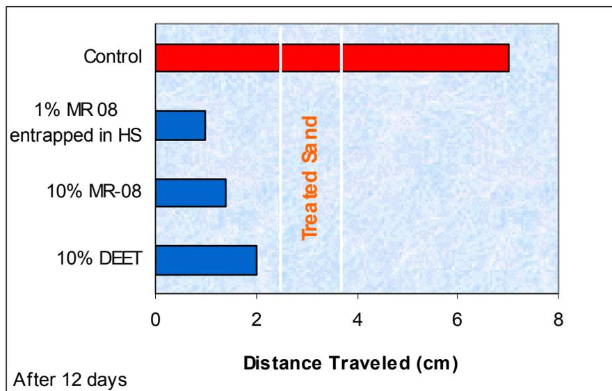
**Fig.4.** Effect of MR-08 against termites in the sand-barrier test. MR-08 is slightly better than DEET when tested. It is significant to note that when MR-08 was entrapped in a microtubule at one tenth the concentration, it produced a more effective inhibition of termite migration compared to the higher concentration of DEET or MR-08. This suggests that slow release technology may contribute to lower requirement of the active ingredient.
