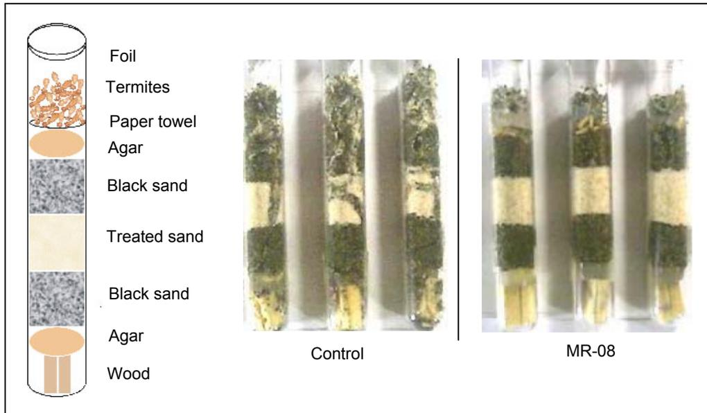
**Fig 3.** Distances traveled by the termites through the sand barrier. In the control group, the termites have reached the wood blocks by day 6 and burrowed to a distance of 7 cm. In MR-08 treated sand barriers, the termites remained stationary at 1 cm and no damage to the wood blocks until the termination of the test on day 12.
