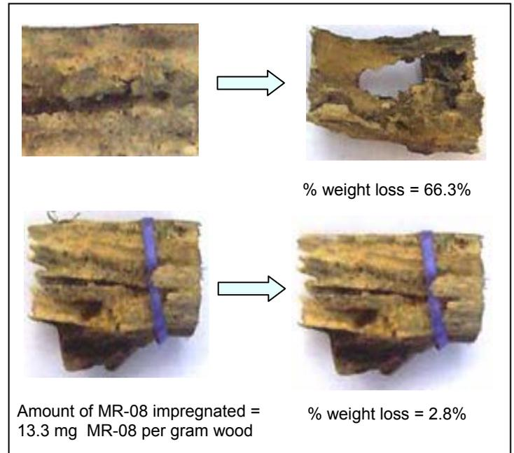
**Fig. 5. Effect of MR-08 on prevention of wood damage by the wood termite (*Coptotermes vastator*). MR-08 was impregnated into the wood overnight using an ethanolic solution and the wood sample placed in a termite mound for 2 weeks.**
