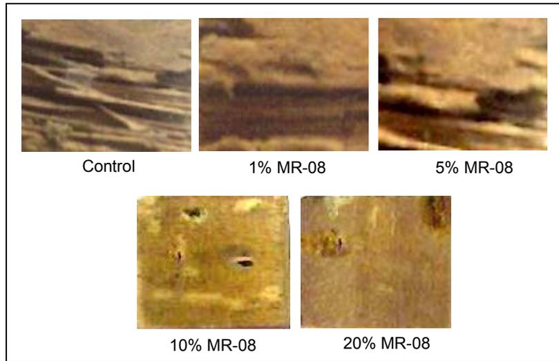
**Fig. 7. Photographs of wood samples at four (4) months after single superficial impregnation of wood with various concentrations of MR-08.**
