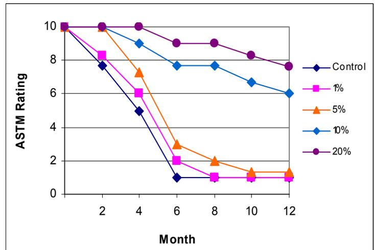
**Fig. 6. The effect of MR-08 at various concentrations in protecting wood substrates against termite damage. Standardized wood samples were impregnated with MR-08 and placed in termite mounds. The samples were taken for evaluation at each month of exposure.**
