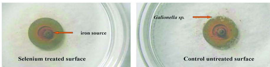
Fig 4. The presence of covalently bound selenium prevents growth of Gallionella sp overgrowth over metallic surface after nine days of immersion in Gallionella rich culture
